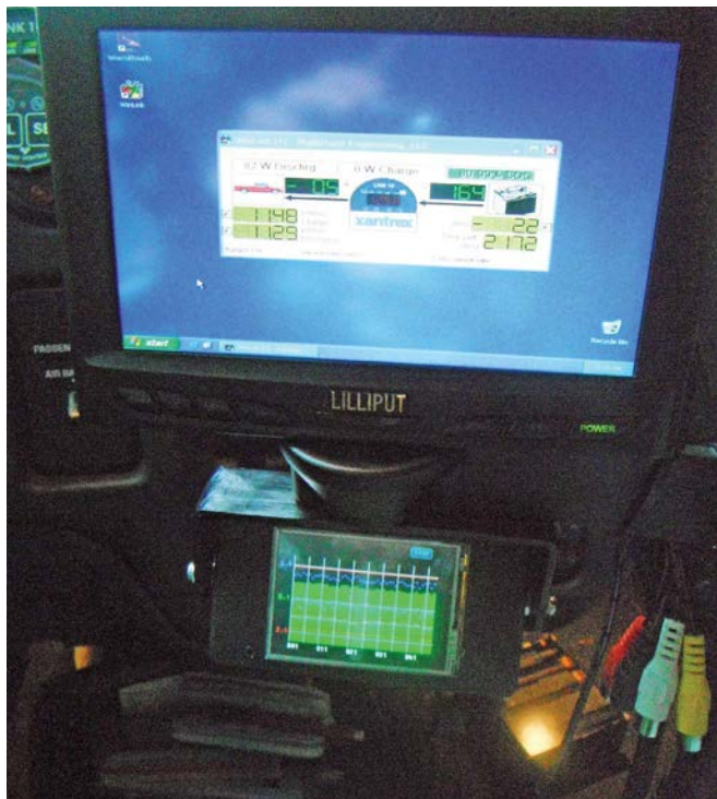
The truck's in-cab battery monitors show battery state-of-charge (top), and BMS cell voltage and temperature (bottom).
