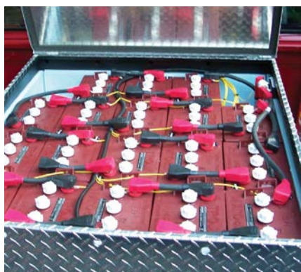
Eighteen of the original FLA batteries in a custom-built box in the truck bed. The six other batteries were housed under the truck’s hood.
